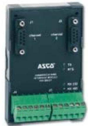
Fig. 16: Communication Interface Module
